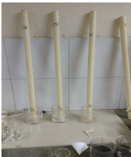
Figure 3. PVC pipes filled with different % sand filtering water
